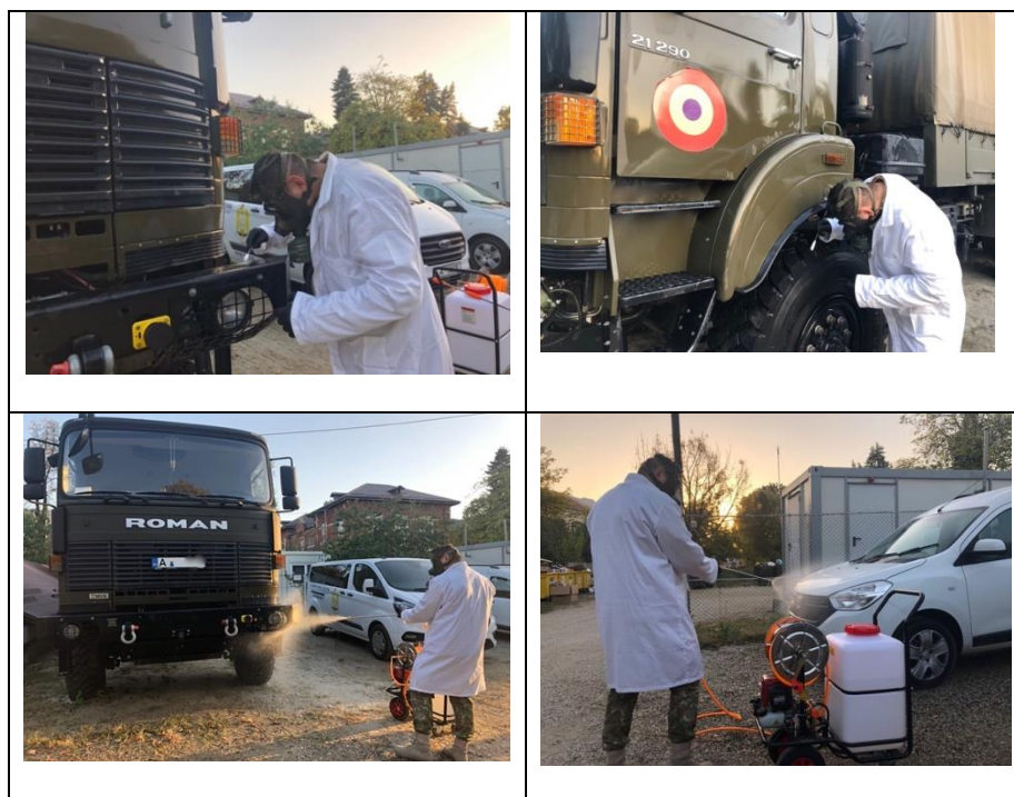
Fig. 4 – The contaminated surfaces and the dispersion of the decontamination solution - NANODEC-RBC on the three types of surfaces - rubber (wheels), hood (painted metal) and metal bar.
